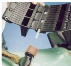
B) Remove Slide-Lock by backing it out, do not pull it through to remove broken piece. Tap broken piece back out.
