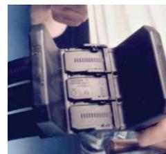
D) If the Slide-Lock does not completely lock into place the following may have occurred. Two or more segments may have engaged completely. To rectify back Slide-Lock out and readjust segments by pulling them apart by hand. Re-insert Slide-Lock and adjust tightness of the spacer with another segment.
