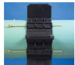
**Note:** Properly installed slide-locks will rarely be driven all the way in. To secure a tight fit drive as far as possible, but if all are driven completely, (bottomed out) it may not be tight enough. Verify Ranger II casing spacer cannot slide on carrier pipe.
