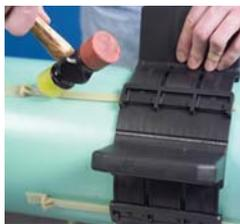
7A. To tighten Ranger II securely to carrier pipe, back Slide-Lock completely out of the slot. If needed, push segments together by hand. **Note:** You may have to release tension by loosening other Slide-Locks.
